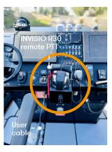
The INVISIO personal system (headset-control unit) provides clear comms and hearing protection. The INVISIO R30 remote PTT allows for handsfree communication.
