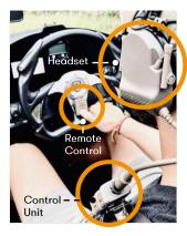
The INVISIO personal system (headset-control unit) provides clear comms and hearing protection. The INVISIO R30 remote PTT allows for handsfree communication.
